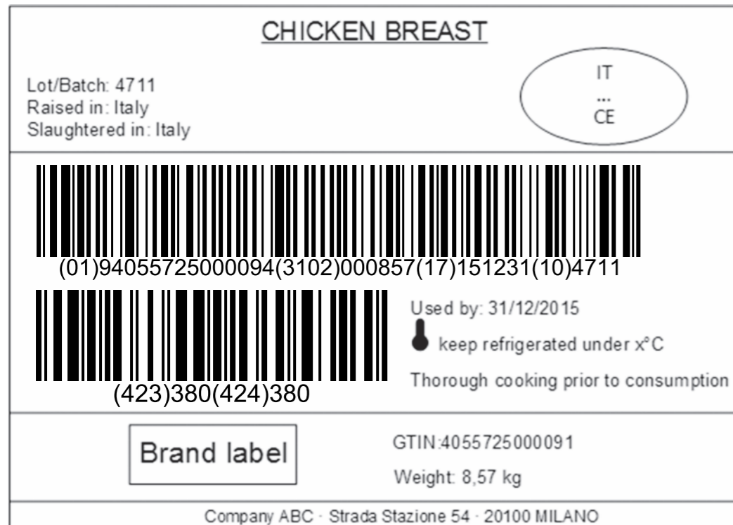
Figure 8 – carton/crate label with GS1-128-barcode
