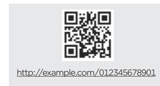
Figure 3 - Example for product URL encoded in a GS1 QR Code
